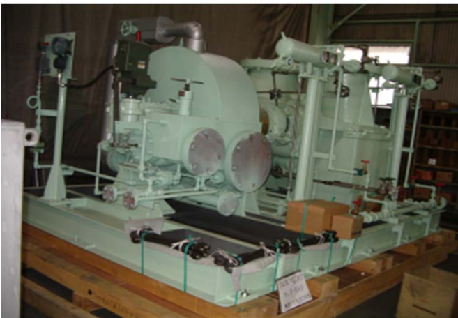
Turbine Driven BB2 Pump
