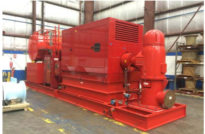
Packaged Fire Pump System
