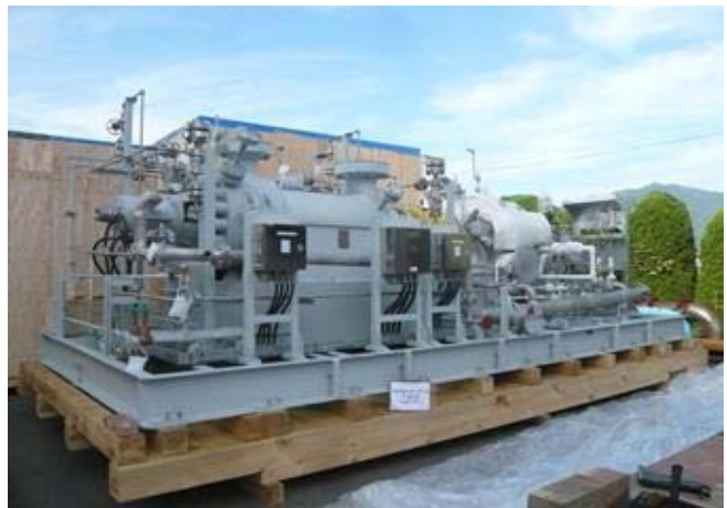
Turbine Driven BB5 Pump
