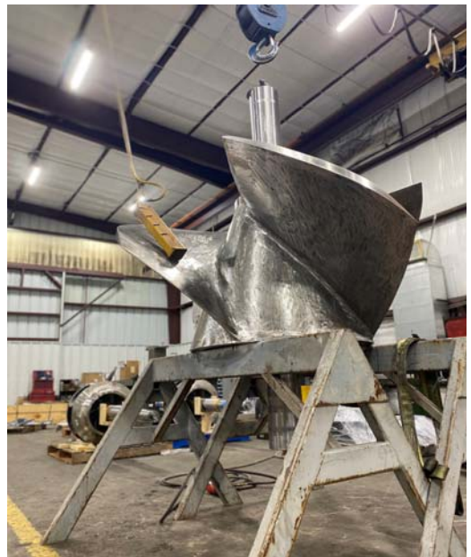
55" Mixed Flow Pump Work
