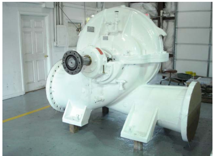
Split Case Pump Repair
