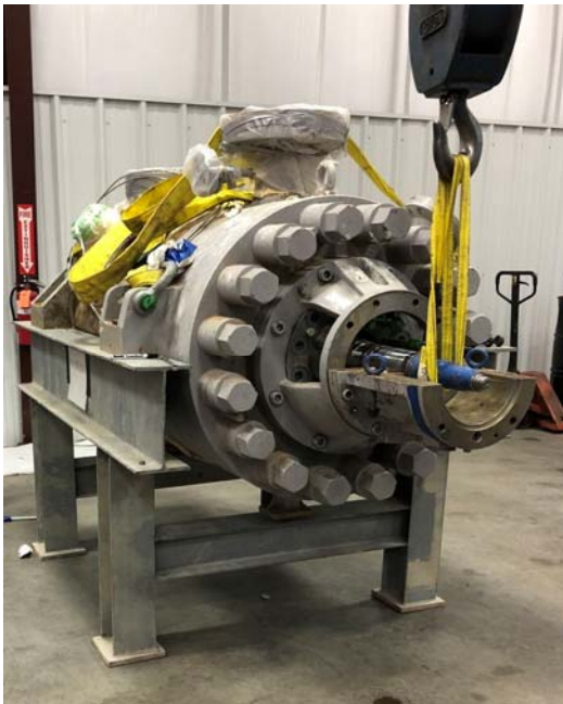
BB5 Repair Work
